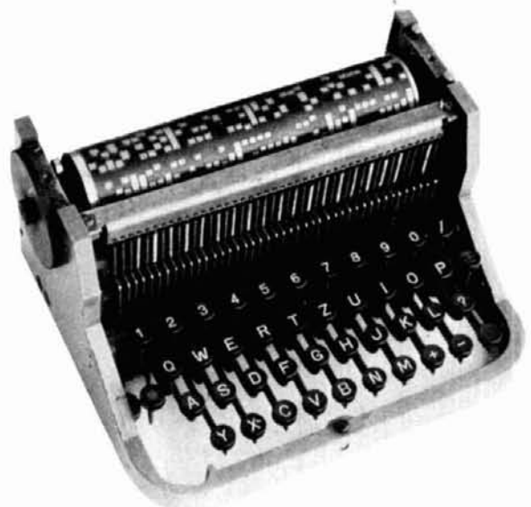
Transmitter section of the original Hellschreiber. The coded drum turns one revolution per character. Every time a key is pressed, one turn of the drum produces a series of pulses by the contact with one series of lamellas.
