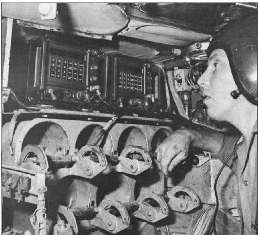
Dual VRM 5080 system installed in a Chieftain main battle tank
