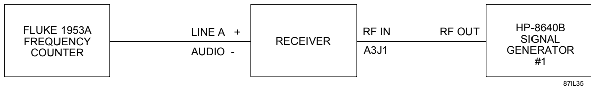
Figure 7-4. Fine Tuning Accuracy Performance Test Equipment Connection
