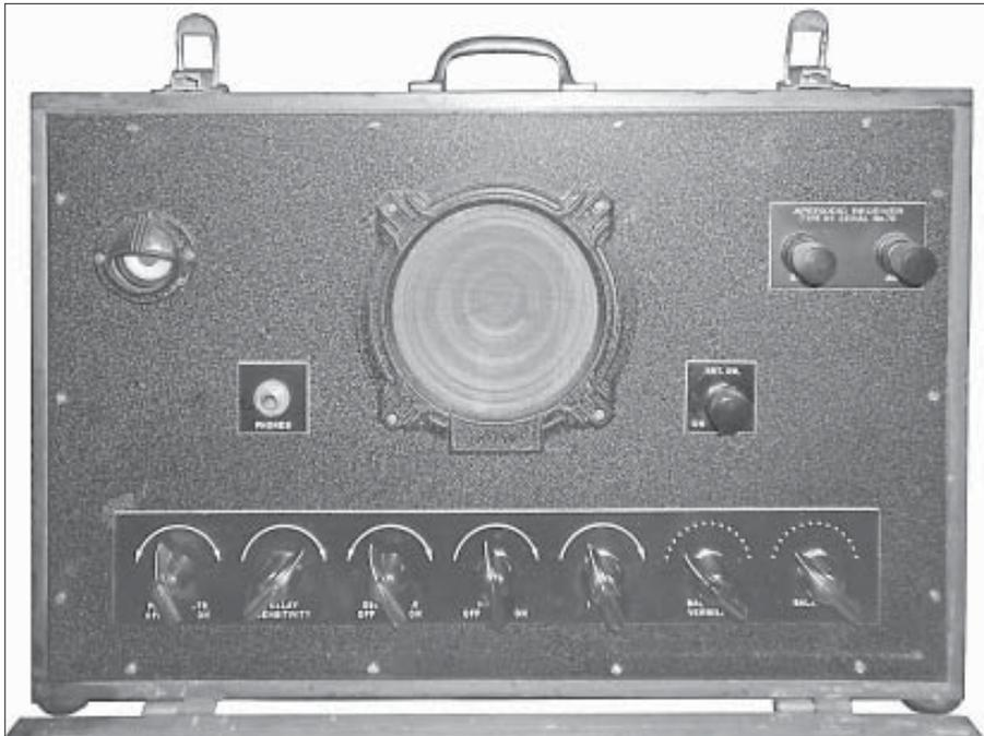
**Figure 3: The SSR-201 receiver used black wrinkle paint and white lettering.**
