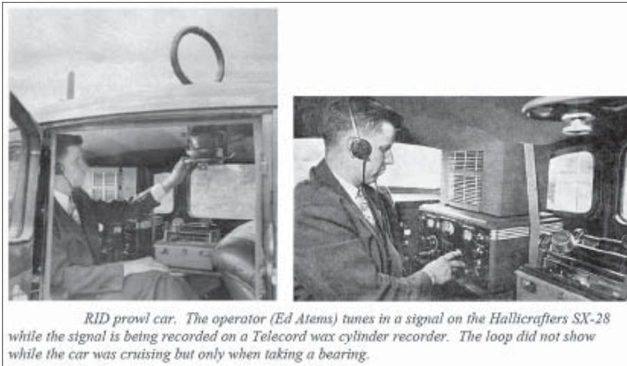
**Figure 5:** This photo of the RID “prowl car” does not show a SSR-201 in use, but the government agents are using the Hallicrafters SX-28 in direction-finding applications with a retractable loop, mounted on the roof of the vehicle. The Hudson Motor Car Company had contracts for some of the FCC radio sedans.
