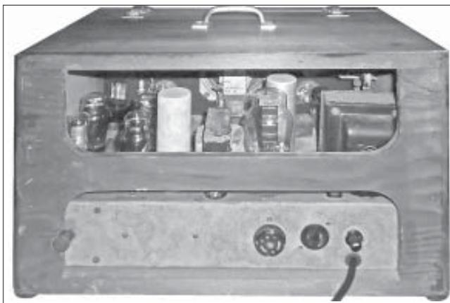
**Figure 4: The SSR-201 was built into a simple blonde-colored wooden case with a hinged front cover.**
