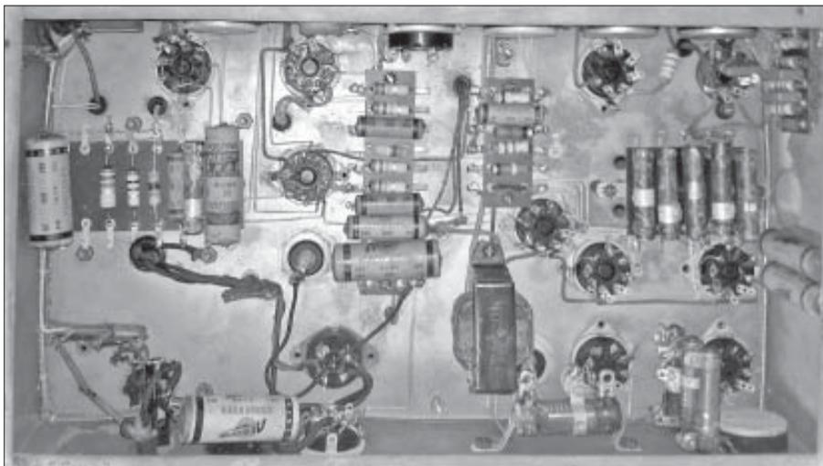
Figure 8: In this below-chassis view of SSR-201, S/N K70, notice the use of “tag” boards (mounting boards) for all of the discrete components, resistors and capacitors, associated with nearby electron tubes.
