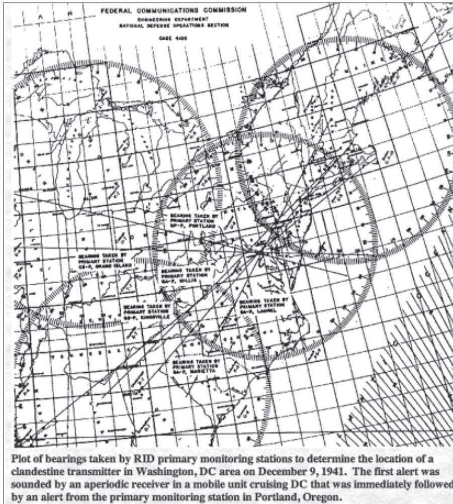
**Figure 5: Direction finding plots were used to pinpoint spy transmissions.**
