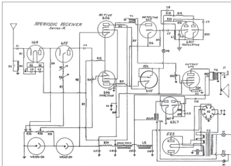
**Figure 6:** This is a schematic for the series-K SSR-201 receiver.
