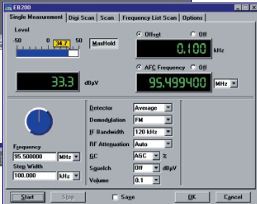
FIG 3 Even single-frequency measurements can be stored and conveniently documented together with all receiver settings
