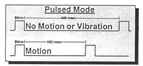
If the auxiliary contact is open, every fourth pulse is doubled in width.
