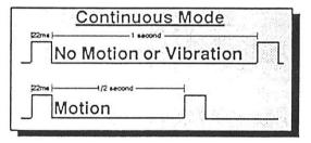
If the auxiliary input contact opens, every fourth "blip" is tripled in width.
