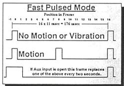
Certain less sophisticated DF equipment may have problems coping with the ordinary pulsed mode of the D903. An option is therefore selectable by the user to allow the fast pulsed mode to be replaced by a pulsed mode with wider pulses. As in normal pulsed mode, this mode changes its pulse repetition rate according to the state of motion:
