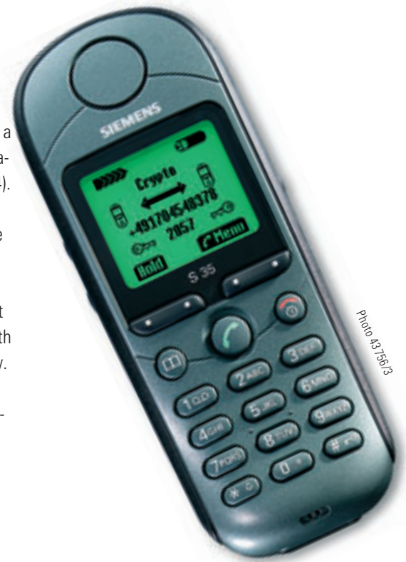
FIG 3 R&S TopSec GSM crypto mobile phone (described in detail in previous issue)
