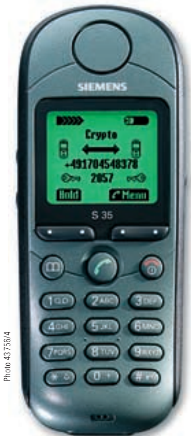
FIG 2 The activated crypto mode is indicated on the display
