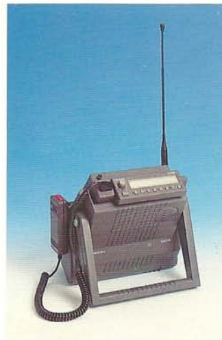
FM1100-PM portable unit in desk top-mode.
