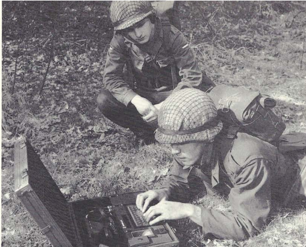
Philips USFA's MINIFLEX compact high-grade crypto system in operation in the field. The lightweight transit case contains a complete terminal, with telephone and radio modems and a miniature printer.
