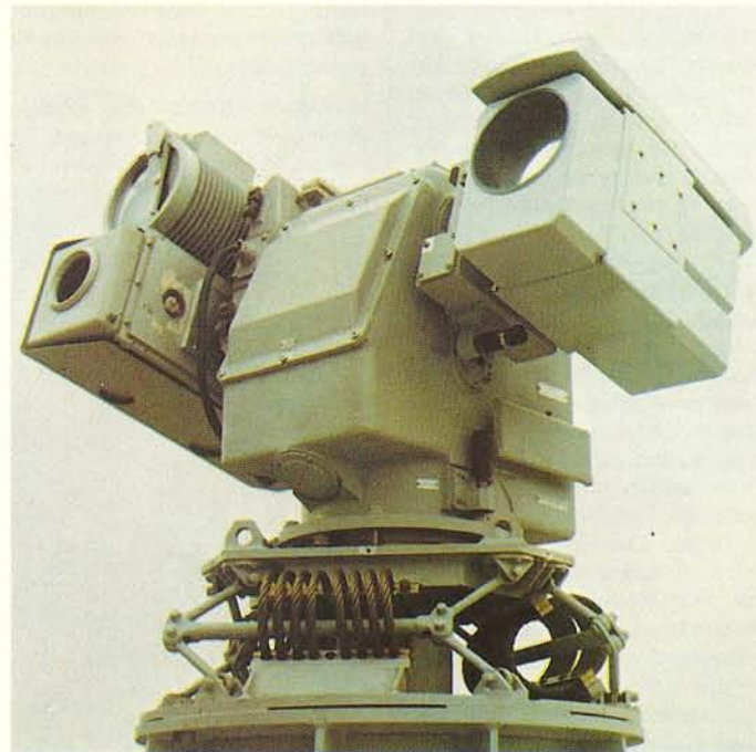
Philips USFA's thermal imaging camera UA9053 mounted on the Hollandse Signaal LIOD electro-optical director system.
