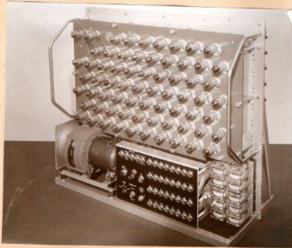
"Philips Hefa Erolet I" type no.Us 8020. Interior (front) with control panel.
