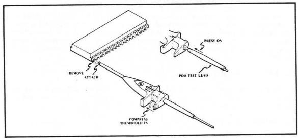
Figure 3-5. Test Terminal Grabber Connections
