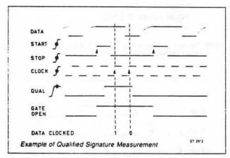
The qualified signatures function is identical to the normal signatures function except that an additional measuring condition (qualifier) is used to select either HIGH or LOW level to enable data to be clocked in.
