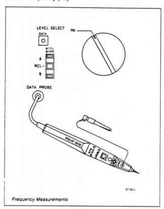
Frequency measurement (Hz) is an automatic function, giving:
