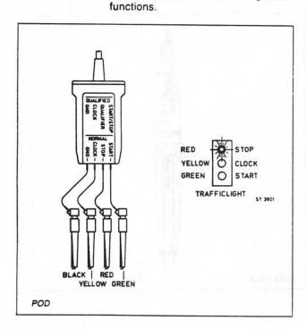
The colour-coded leads of the POD can be easely identified when connecting into logic circuits by use of a 'traffic-light' mnemonic.
