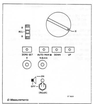
Measured with the test leads connected to V- $\Omega$ -mA and 0 front panel sockets.
