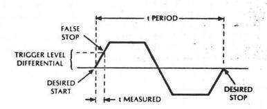
For Time Interval measurements, the expected result would be the period (t period) of the input sinewave. However, depending on the trigger level differential, an unexpected measurement (t measured) may result.
