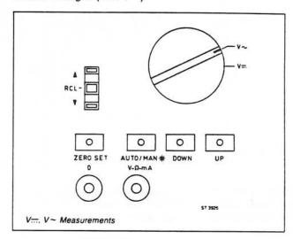
Measured with the test leads connected to V- $\Omega$ -mA and 0 front-panel sockets.
