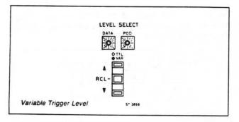
When the default data is displayed, by depressing the midposition of the RCL pusbutton as shown above, this may be varied between - 12.7 V and + 12.7 V by means of the and ends of the RCL pushbutton.
