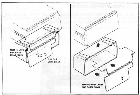
Figure 3-3. Front Panel Storage Cover Removal
