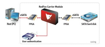
The diagram above illustrates the concept of a transparent eSATA hard disk encryption device that is 'seen' by the host as a normal hard disk. The RF-CM is placed in the SATA data path. Surrounding FPGAs encapsulate eSATA frames in Ethernet frames, and vice versa. Two separate FPGAs are used to guarantee the red-black separation. The hardware fast-path is programmed to encrypt or decrypt the eSATA frames inside the Ethernet frame's payload at high speed.
