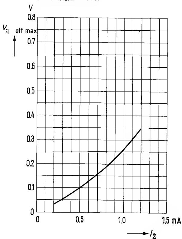
**Voltage gain v. current  $I_2$**  $V_{cc} = 1.3 \text{ V}, R_L = 500 \Omega,$  $f = 1 \text{ kHz}$
