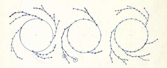
Here, each wheel position is denoted by a dot, and the arrows lead from each position to it's immediate successor.
