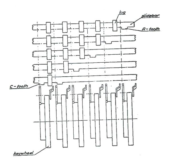
Placement of Lugs on Bars Controlling Motion, CX-52M
